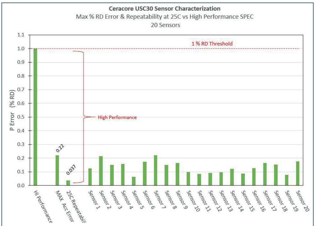
Figure #11: Standard Pressure Sensor Accuracy vs Ceracore USC30 Accuracy plotted as % RD
