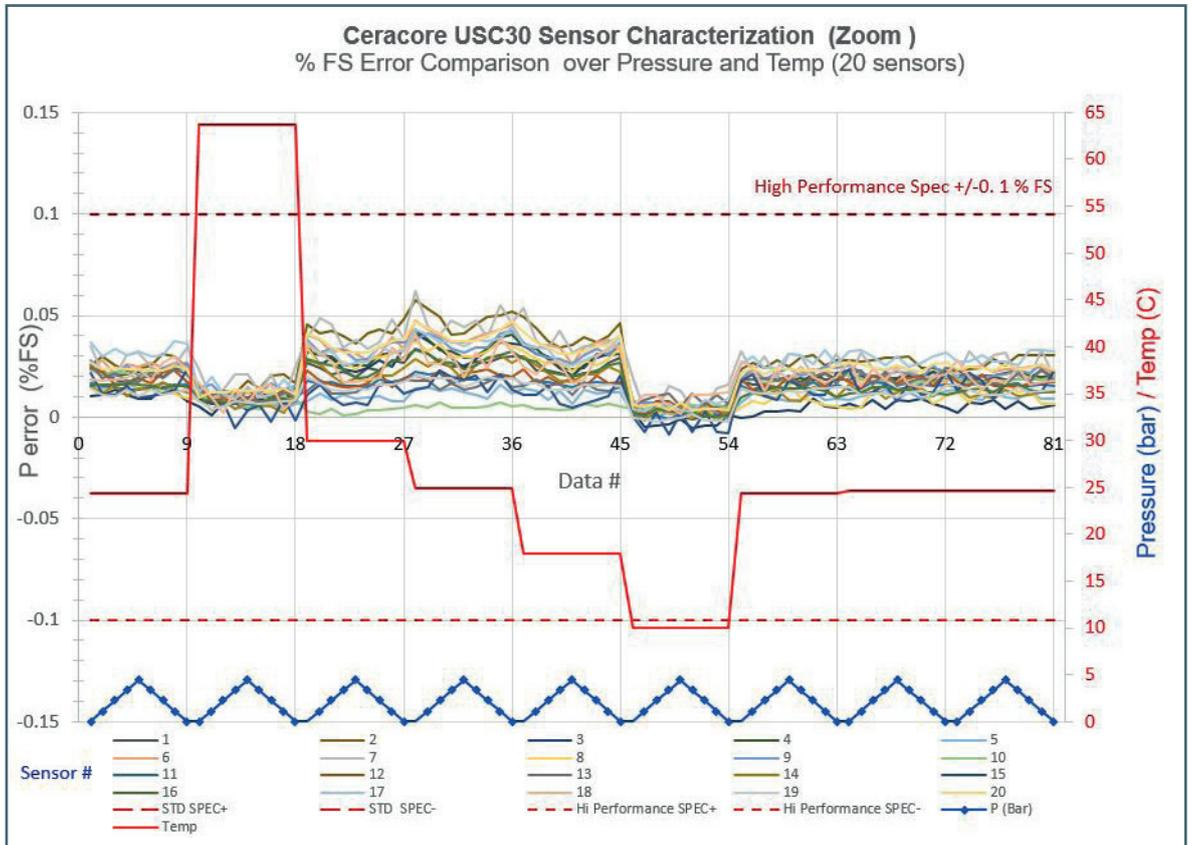
Figure #4: Pressure and Temperature Verification Result for 20 Ceracore USC30 Sensors. Zoomed in accuracy plotted in % FS.
