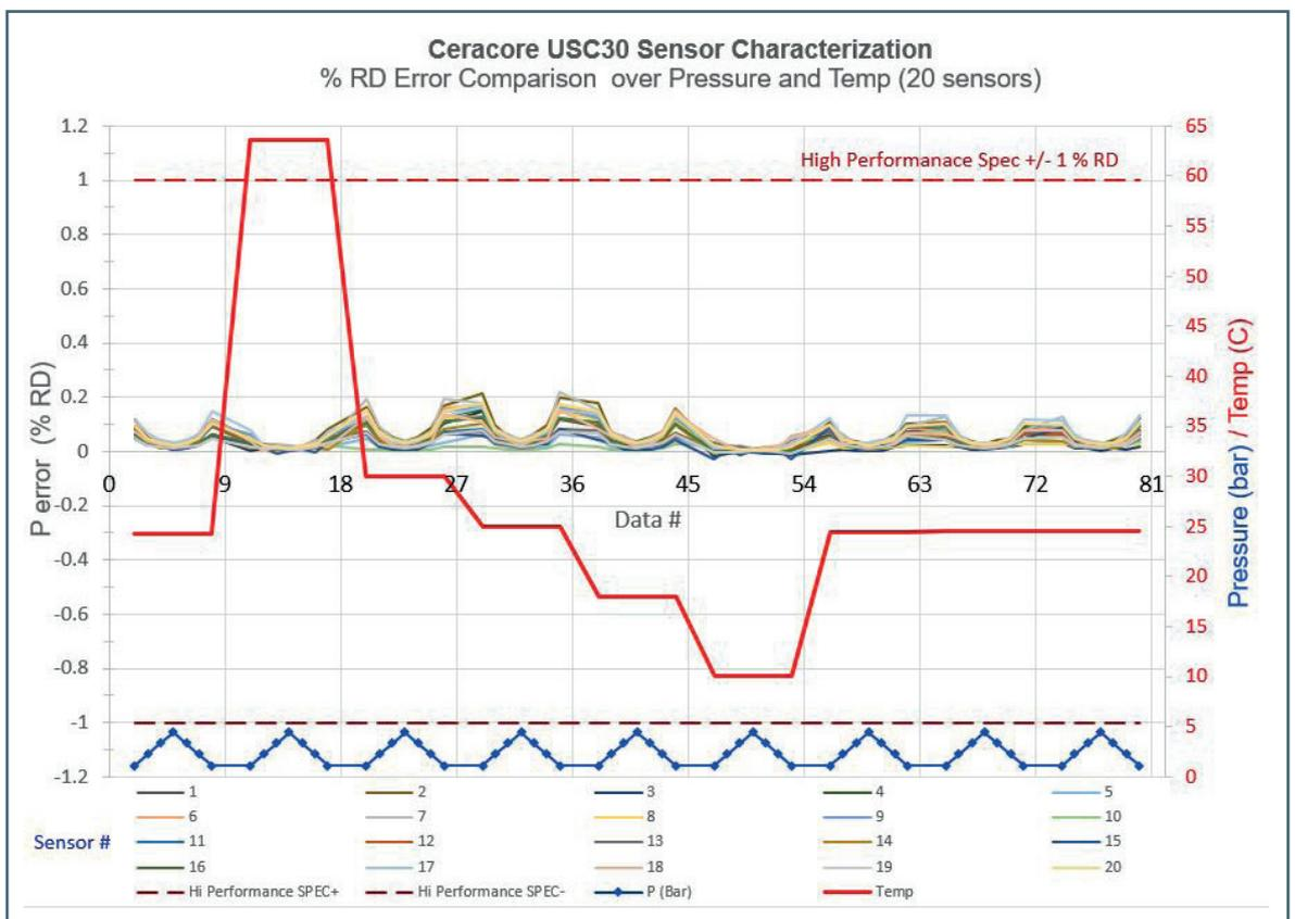
Figure #8: Pressure and Temp Verification Result (% RD Error) for 20 Ceracore USC30 Sensors
