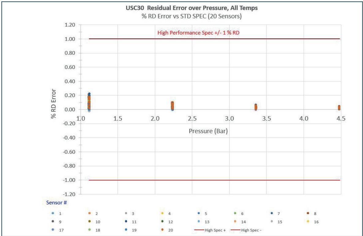
Figure #9: Pressure Effects of USC30 Sensors. % RD Error vs Pressure for all Sensors
