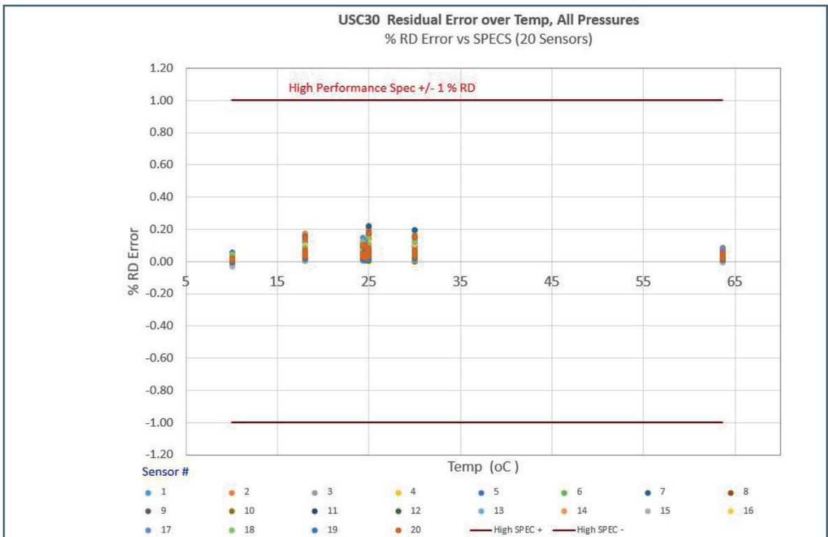
Figure #10: Temperature Effects of USC30 Sensors. % RD Error vs Temperature for all Sensors
