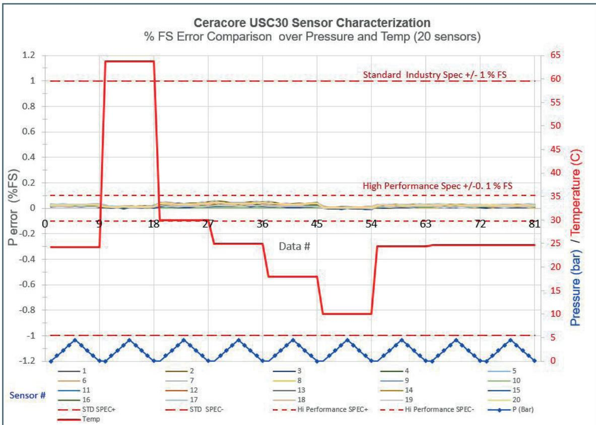
Figure #3: Pressure and Temp Verification Result (%FS%) for 20 Ceracore USC30 Sensors
