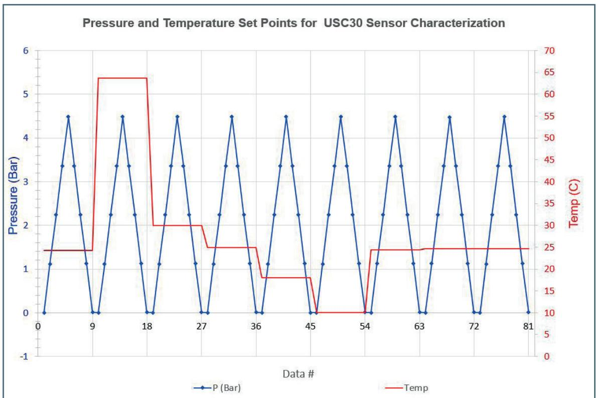
Figure #2: Pressure and Temperature Verification Sequence
