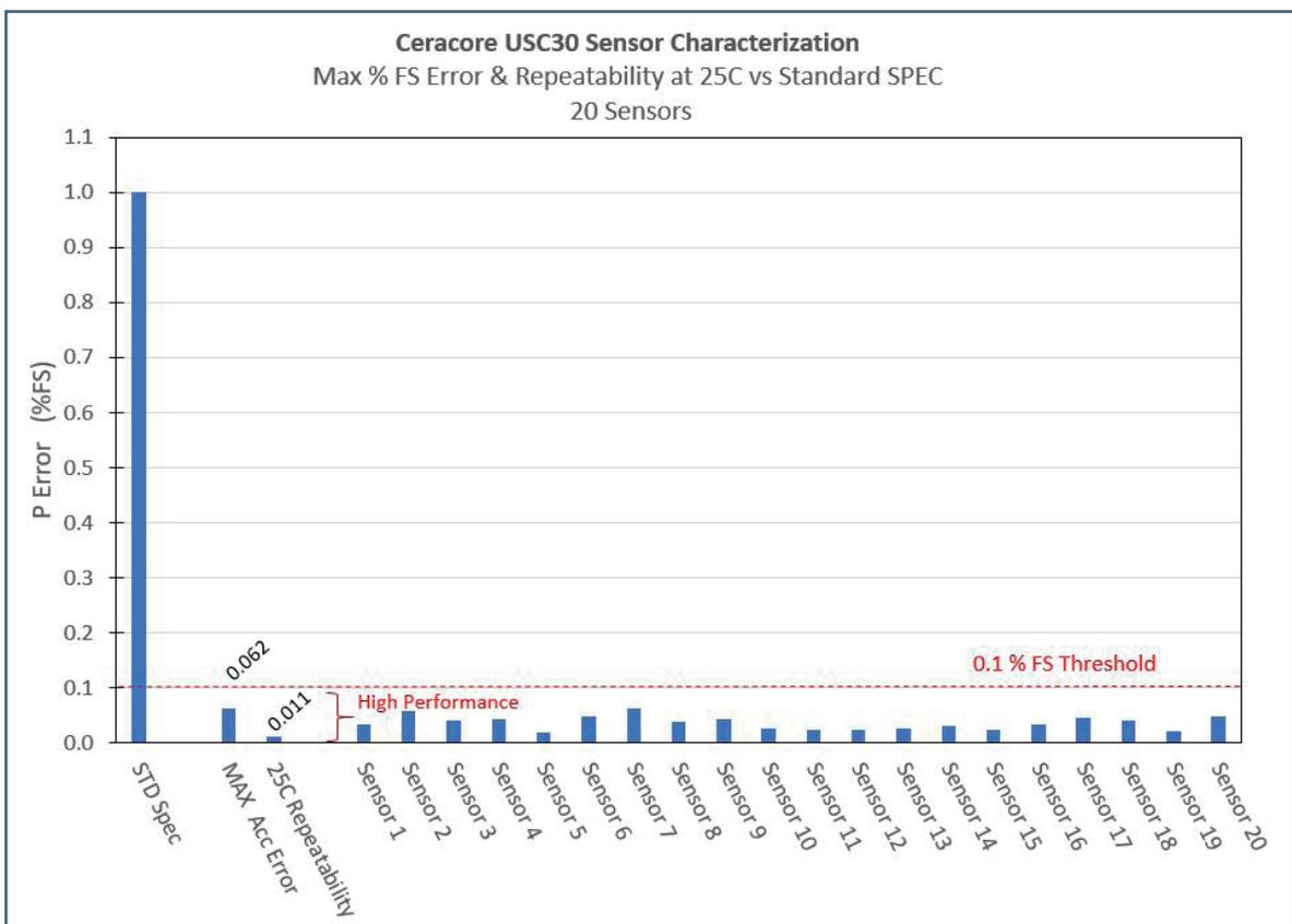
Figure #7: Summary of all Sensors. Max % FS error accuracy @ all temps and repeatability at 25°C
