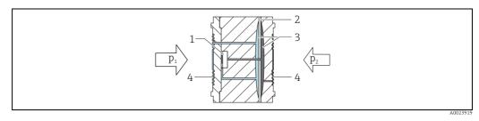
Measuring element Overload diaphragm 1 2
